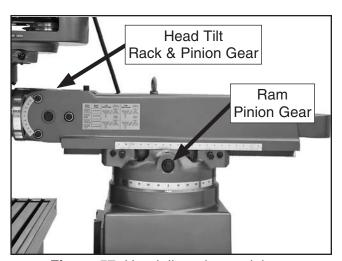
Figure 57. Head tilt and ram pinions.
